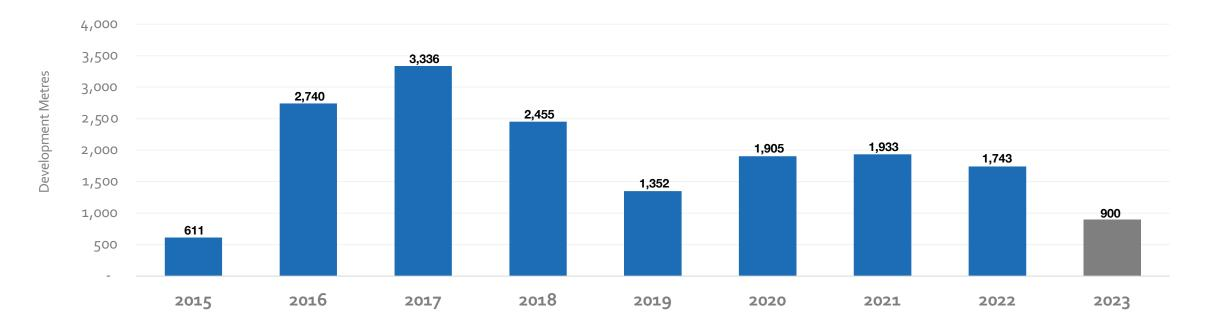
Values above the bar are the total number of metres of adit development for production and exploration purposes at the Pinargozu Zinc Mine. 2023 data is a projection. During Q3, Horzum AS completed 293 metres of both horizontal and inclined development were completed.
