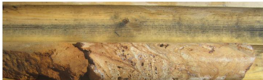
Silty Limestone, Strongly Invaded by Mineralized Veinlets and Replacements. Locally Gossanous. Hole GD-10 at 177 Feet
