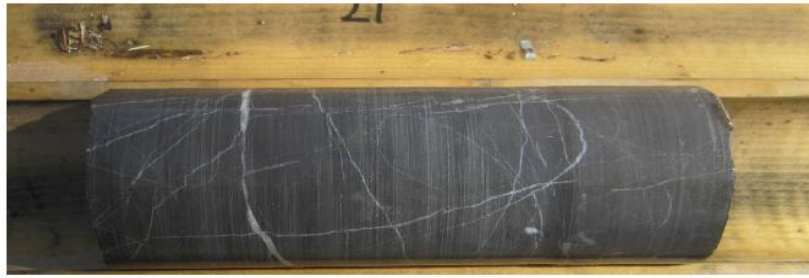
Silty Limestone, Unaltered. Hole GD-10 at 27 Feet
