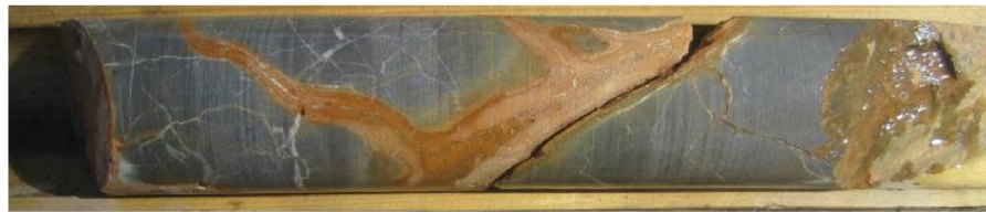
Silty Limestone, Mineralized Veinlets Invading Fractures . Hole GD-10 at 172 Feet
