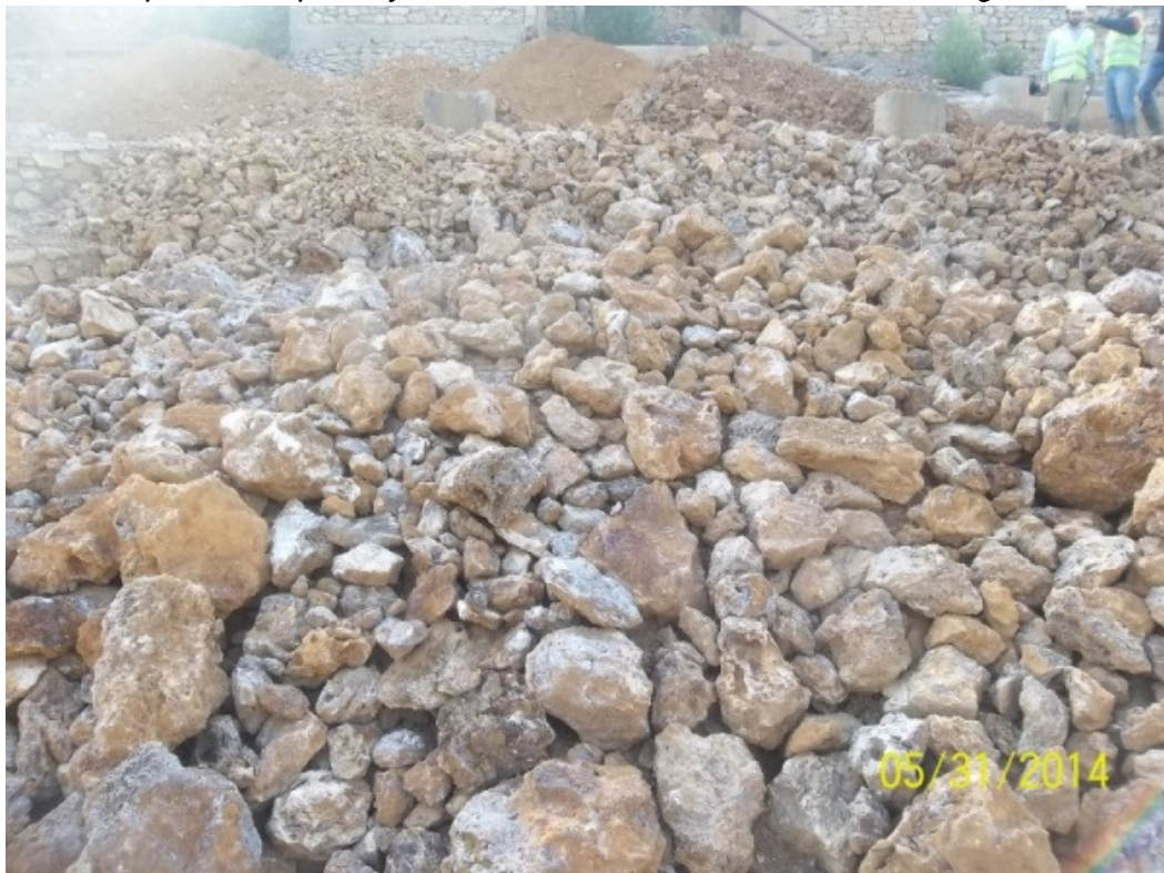
Piles of sulphide Zn (reportedly at 27% Zn) and lead from Horzum and Pinargozu
