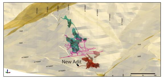
Figure 1 – Schematic showing underground workings relative to the mineralization halo. The adit indicated in red is the new adit.
